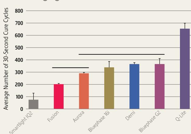
Vertical bars and error bars represent the mean and standard error of the mean, respectively, based on three specimens for each of three units (see statistical note, p. 3). Horizontal bars represent products that are not statistically different (one-way ANOVA followed by the Student-Newman-Keuls method for multiple comparisons,  $p > 0.05$ ).
