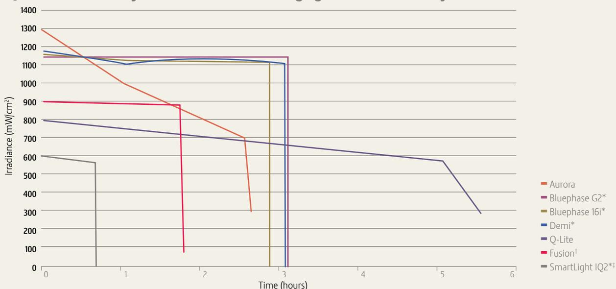
\* Light shut itself off at the point where the curve sharply drops to zero.
