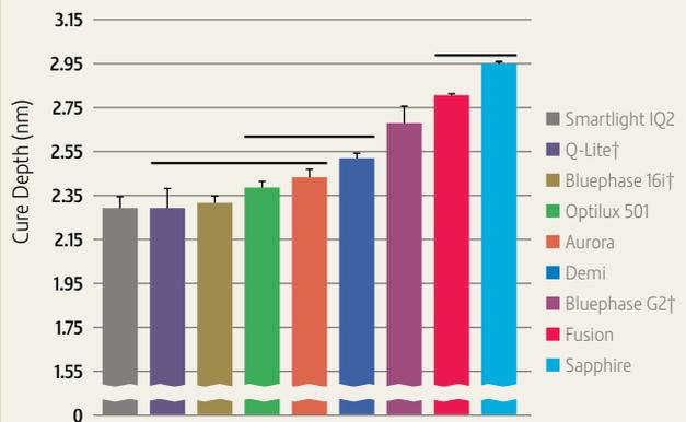
Mean depth of cure and standard error of the mean for each light is shown (n=3 based on three specimens for each of three units). Horizontal bars represent products that are not statistically different (Two-way ANOVA followed by the Bonferroni *t*-test for multiple comparisons,  $p < 0.05$ ).
