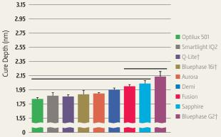
Mean depth of cure and standard error of the mean for each light is shown (n=3 based on three specimens for each of three units). Horizontal bars represent products that are not statistically different (Two-way ANOVA followed by the Bonferroni *t*-test for multiple comparisons, p < 0.05).
