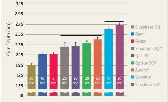
Mean depth of cure and standard error of the mean for each light is shown (n=3 based on three specimens for each of three units). Curing time for each light is indicated in its respective bar. Horizontal bars represent products that are not statistically different (Two-way ANOVA followed by the Bonferroni *t*-test for multiple comparisons, p < 0.05).
