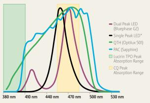
\* This is a representative curve for the single-peak LED curing lights: the Aurora, Bluephase 16i, Demi, Fusion, Smartlite IQ2, and the Q-Lite all have the same shape but with different peak wavelengths, effective spectral range and full spectral range. See Table 2 and Figure 5 for a comparison of these parameters among the different LED curing lights.
