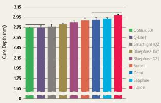
Mean depth of cure and standard error of the mean for each light is shown (n=3 based on three specimens for each of three units). Horizontal bars represent products that are not statistically different (Two-way ANOVA followed by the Bonferroni *t*-test for multiple comparisons,  $\rho < 0.05$ ).
