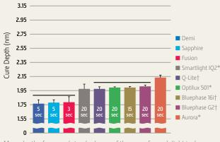
Mean depth of cure and standard error of the mean for each light is shown (n=3 based on three specimens for each of three units). Curing time for each light is indicated in its respective bar. Horizontal bars represent products that are not statistically different (Two-way ANOVA followed by the Bonferroni *t*-test for multiple comparisons, p < 0.05).
