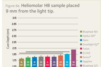
**0** Mean depth of cure and standard error of the mean for each light is shown (n=3 based on three specimens for each of three units). Curing time for each light is indicated in its respective bar. Horizontal bars represent products that are not statistically different (Two-way ANOVA followed by the Bonferroni *t*-test for multiple comparisons, p < 0.05).
